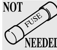
Even if voltage is mistakenly applied to the resistance range, the internal excessive voltage protection element (PTC thermister) protects the circuits for up to 600 V AC.
