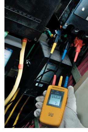
The phase rotation indicator is a handheld instrument designed to detect the rotary field of three-phase systems.
